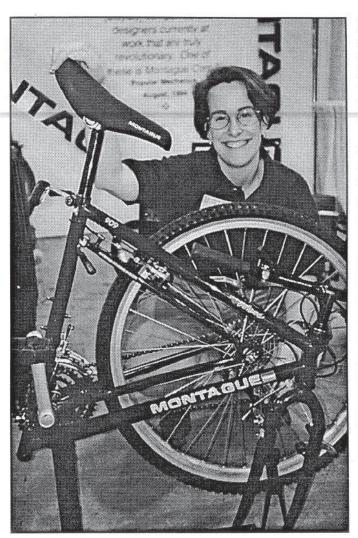
Fold, UNFOLD. Fold, UNFOLD. Kate Stockwell (left) demonstrated Montague folding bicycles to thousands of Midwest Bike Show visitors. Montague bicycles rely on a concentric seat tube design (one tube inside the other) for its quick, "look-ma-no-tools" folding act. Mountain bike versions fold to approximately 3'x3'x1'.
